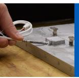
Taken from an embedded RTD probe for accurate readings, accuracy within 3-5° from the setting
