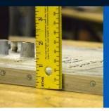
1" thick platen with cast-in heating maintains the heat
